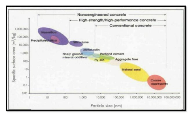
Fig .1 particle -size and specific -surface-area related to concrete materials [3]
