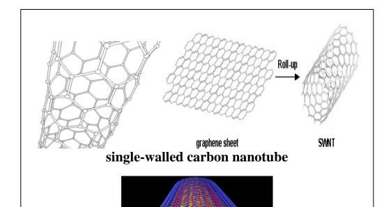
Fig .2 single-walled carbon nanotube and Multi-walled carbon nanotube [8]
