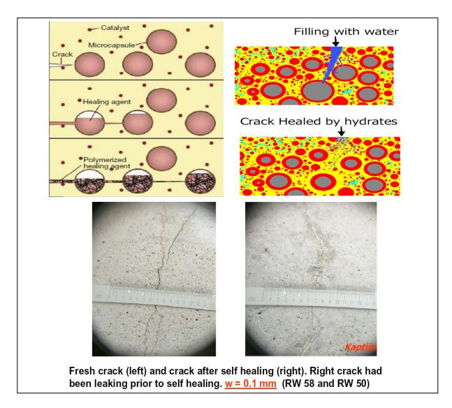
Fig. 5: Mechanism of self healing concrete [15]
