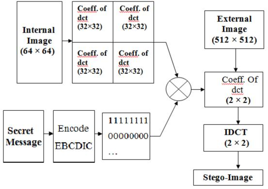
Figure 1 block diagram represent the insertion algorithm
