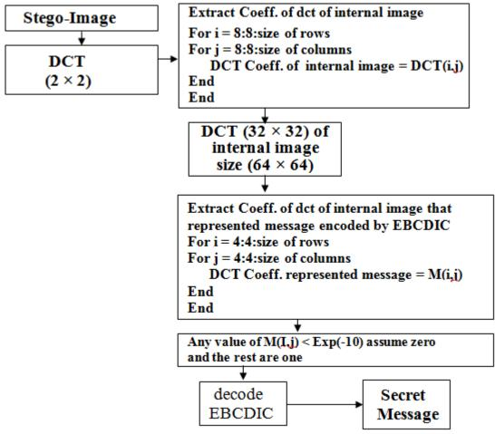
Figure 2 block diagram represent the detection algorithm
