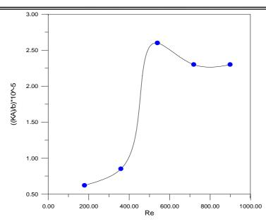
Figure 3 Effect of Re number on mass transfer coefficient
