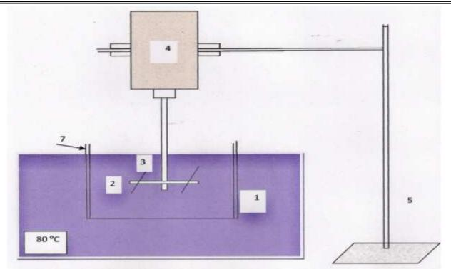
**Figure 1** A Schematic diagram of the experimental apparats 1-Glass reactor, 2- Impeller, 3- Shaft, 4- Motor, 5- Stand, 6- Water bath, 7-baffle
