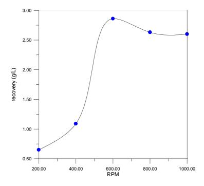
Figure 2 effect of agitation speed on nickel recovery at T=80 °C
