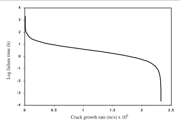
Fig.3: The time to failure (t<sub>f</sub>) Vs. crack growth rate (V) at stress ratio of 0.64
