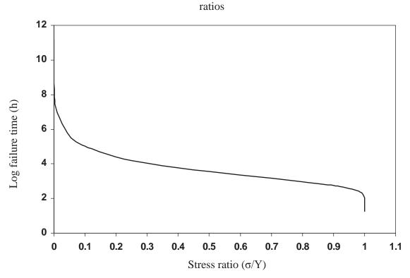
**Fig.2:** The time to failure  $(t_f)$  Vs. stress ratio  $(\sigma/Y)$
