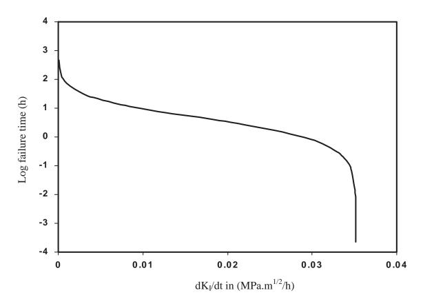
Fig.4: The time to failure ( $t_f$ ) Vs. Stress intensity factor changing rate at stress ratio ( $\sigma/Y$ ) of 0.64
