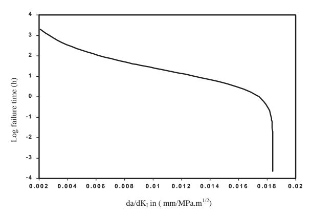
Fig.5: The time to failure  $(t_f)$  Vs. crack growth changing with stress intensity factor at stress ratio  $(\sigma/Y)$  of 0.64
