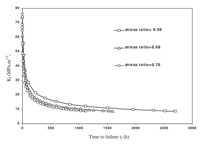
**Fig.1:**  $K_I Vs.$  time to failure  $(t_f)$  plots for current analysis system with different stress
