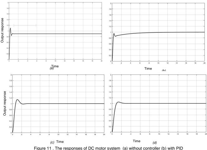
controller (c) with FGA-PID (d) with PSO-FGA-PID
