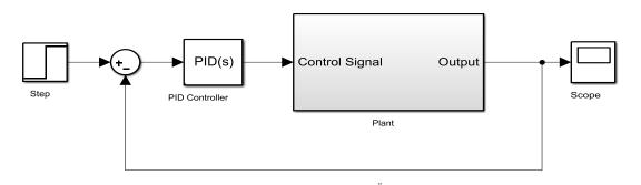
Figure 4. Block diagram of feedback control system with a PID controller simulated by Matlab-Simulink
