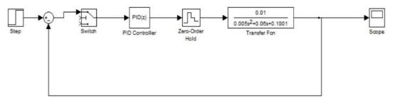
Figure 10. Feedback DC motor control system simulated in Matlab simulank
