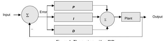
Figure 1. The system with a PID
