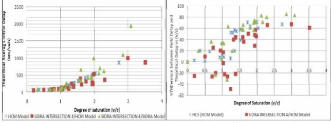
Figure (16) Theoretical delay calculated by the three models according to degree of saturation
