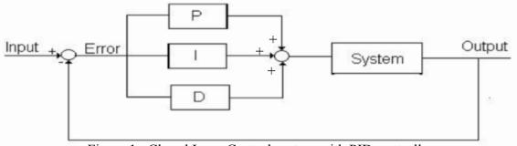
Figure 1 : Closed Loop Control system with PID controller
