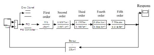
Figure 4: Fifth Order plant with sensor and PID Controller block diagram
