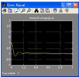
Figure 9: Error Signal of Terminal Voltage Step Response for Fourth Order Model with PID controller
