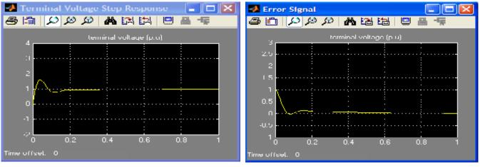
Figure 9 : Terminal Voltage Step Response for 5th Order Model with GPID
