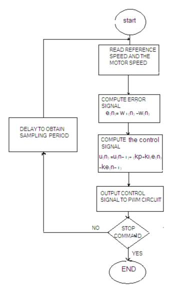
Fig.(5) The software flowchart of speed control.
