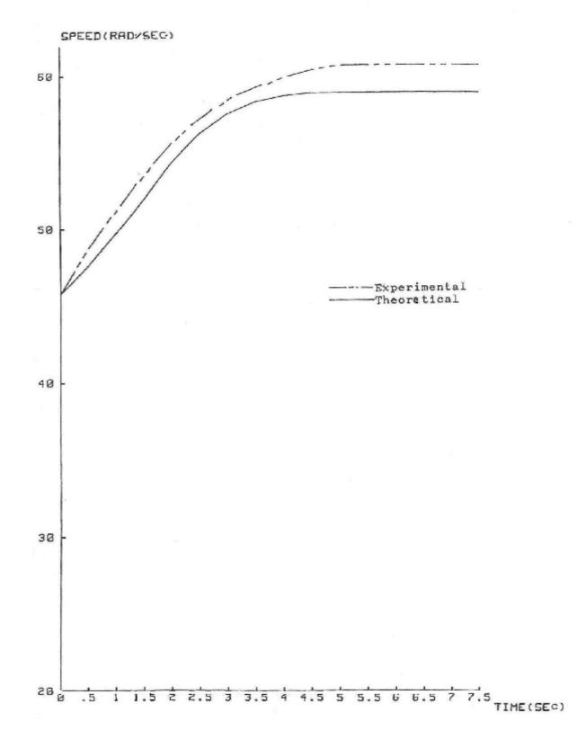
Fig.(8) Experimental and theoretical closed loop transient response of the speed for step change in reference speed Wr from 46.0 rad/sec to 59.3 rad/sec ,  $W_{avo} = 46.0 \text{ rad/sec}$  ,  $i_{vao} = 3.05 \text{A}$ .
