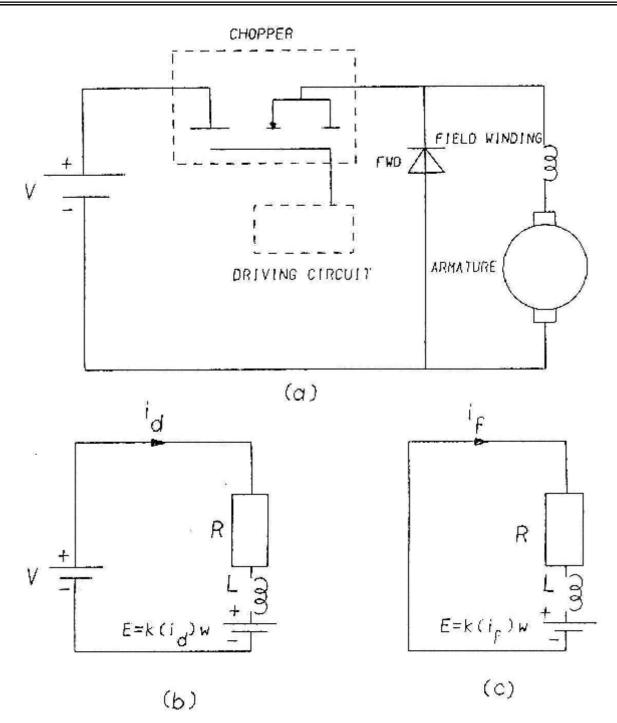
Fig.(2) Representation of a chopper – controlled dc series motor.
