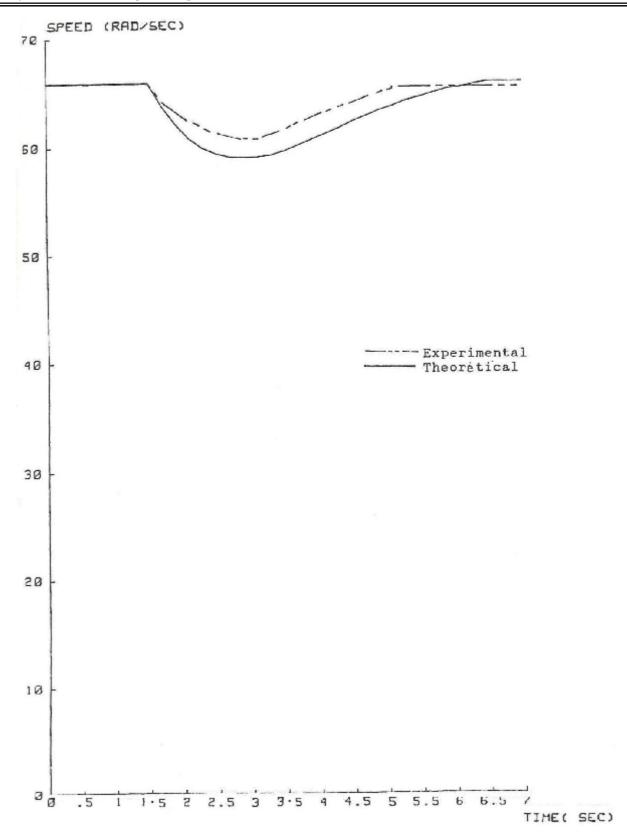
Fig.(6) Experimental and theoretical closed loop transient response of the speed for step change in load resistance RL from  $100^{\circ}$  to  $50^{\circ}$ ,  $w_{avo} = 66.6$  rad/sec.,  $i_{avo} = 2.7$ A.
