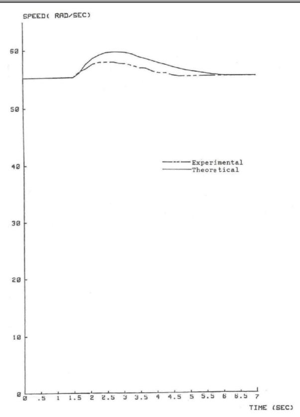
Fig.(7) Experimental and theoretical closed loop transient response of the speed for step change in load resistance RL from 50  $\Omega$  to 100  $\Omega$ , W<sub>avo</sub> = 55.2 rad/sec., i<sub>avo</sub>= 3.38A.
