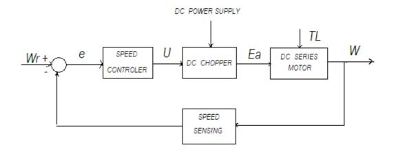
Fig.(3) Block diagram of a closed - loop fed dc series motor.
