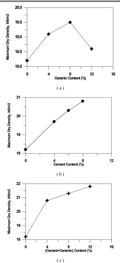
Figure (5):Effect of Additives on Maximum Dry Density. (a) Ceramic, (b) Cement, (c) Cement and Ceramic.
