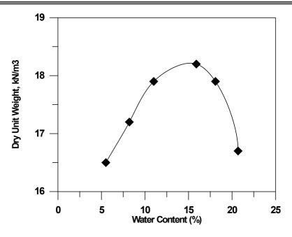
Figure (1): Standard Compaction Curve for Untreated Soil.
