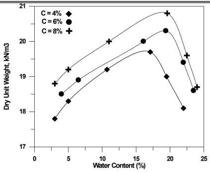
Figure (3): Standard Compaction Curves for Soil Treated with Cement.
