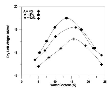
Figure (2): Standard Compaction Curves for Soil Treated with Ceramic.
