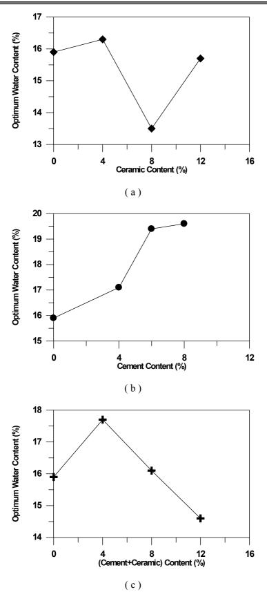
Figure (6): Effect of Additives on Optimum Water Content. (a) Ceramic, (b) Cement, (c) Cement and Ceramic
