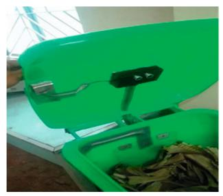
Figure 9. Smart Bin with ultrasonic sensor equipped at surface level
