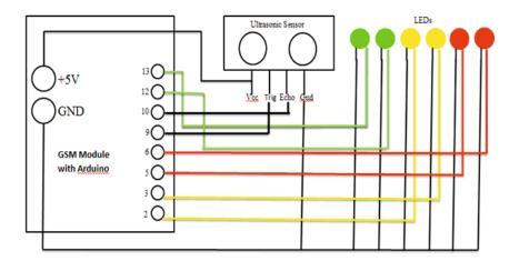
Figure 7. GSM Module with Arduino Ultrasonic Hardware Connection
