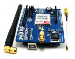
Figure 2. GSM Module SIM900
