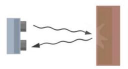
Figure 3. Diagram of the basic ultrasonic sensor operation
