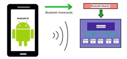
Figure 8. Automatic Lighting System Block diagram
