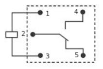
Figure 12. Relay pin-out
