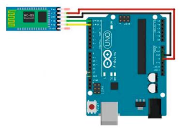
Figure 9. Arduino Bluetooth hardware Connection
