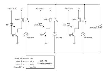
Figure 10. Lighting System Schematic Diagram
