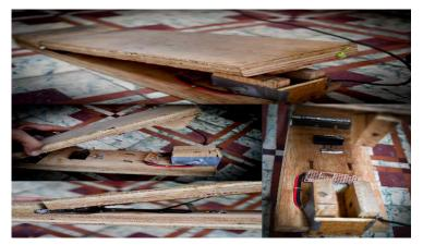
Figure 7. Hi-Hat Trigger Pedal
