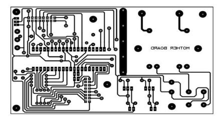
Figure 5. Motherboard Printed Circuit Board
