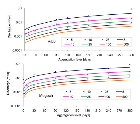
Figure 6. Probabilistic QDF models of Ribb [1961-2004] and Megech (1980-2006)
