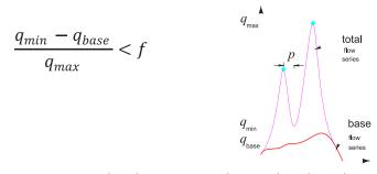
Figure 2. Parameters used in the criteria to select nearly independent extremes from the discharge series (Source: Willems, 2009).
