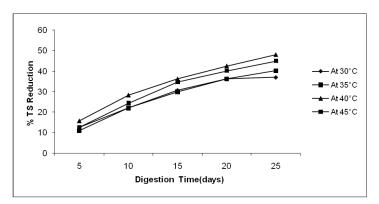
Figure 4. Effect of digestion time on percentage TS Reduction at four different temperatures
