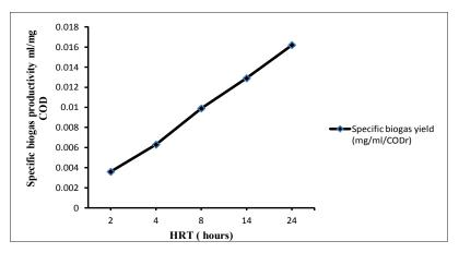
Figure 9. Effect of hydraulic retention time on specific biogas productivity
