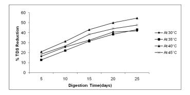
Figure 5. Effect of digestion time on percentage TDS Reduction at four different temperatures
