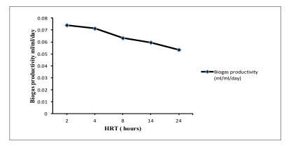
Figure 8. Effect of hydraulic retention time on biogas productivity
