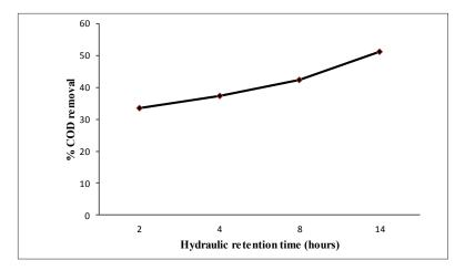
Figure 7. Effect of hydraulic retention time on percentage COD reduction
