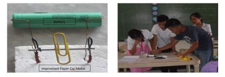
Figure 4. Fourth year students performing the activity in Electromagnetism using the Improvised Electric Motor Model
