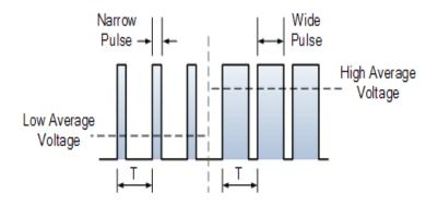
Figure 6. Pulse Width Modulated Waveform
