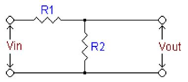
Figure 7. Voltage divider network of the Spark Plug and Ignition Coil Testing Instrument
