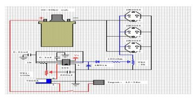
Figure 3. Ignition Coil Driver by Seltzman
