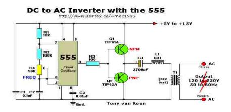
Figure 5. DC to AC Inverter by Roon
