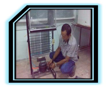
Figure 5. The developed refrigerator trainer
