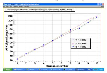
Figure 5. Air column length vs number of harmonics for stopped-pipe using frequencies  $f_1 = 412$  Hz,  $f_2 = 414$  Hz and  $f_3 = 416$  Hz, respectively.
