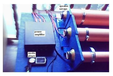
Figure 3. Project accessories: power amplifier, speaker setups and MP3 player.
