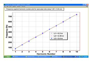
Figure 6. Frequency vs number of harmonics for open-pipe using air column lengths  $L_1 = 2.3$  m,  $L_2 = 2.35$  m and  $L_3 = 2.4$  m, respectively.
