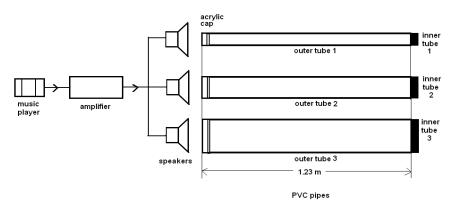
Figure 1. Block diagram of the modified resonator tube apparatus.
