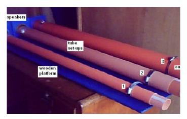
Figure 2. Fully-operational modified resonator tube apparatus.
