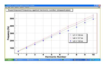
Figure 7. Frequency vs number of harmonics for stopped-pipe using air column lengths  $L_1 = 1.6$  m,  $L_2 = 1.7$  m and  $L_3 = 1.8$  m, respectively.
