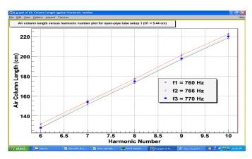
Figure 4. Air column length vs number of harmonics for open-pipe using frequencies f1 = 760 Hz, f2 = 766 Hz and f3 = 770 Hz, respectively.
