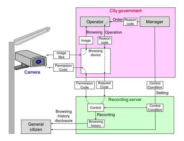
Figure 1. Example of a system based on the concept of abuse prevention of a street camera network by browsing-history disclosure
