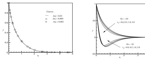
Fig. 2: Velocity profiles for different step sizes
