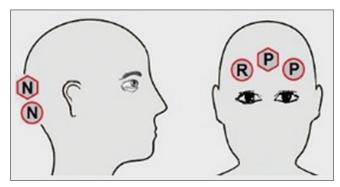
Figure 5: Placement of electroencephalogram electrodes around the head. Circles are wet electrodes, hexagons are active electrodes. "P" and "N" represent positive and negative electrodes, respectively, and "R" is the reference electrode
