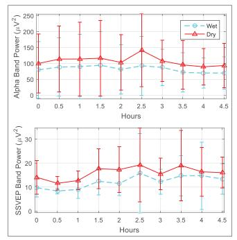
Figure 8: Comparison of alpha waves and steady state visual evoked potentials band power between the electrodes in the long-term electroencephalogram test. The bars demonstrate average and standard deviation of values from five participants during the experiment
