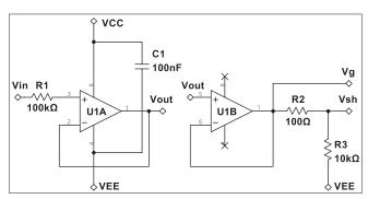
Figure 2: Schematic of the developed active electrode. Vg and Vsh were used for active guarding/shielding of the circuit and output cable, respectively
