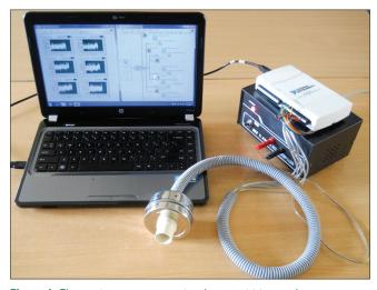
Figure 1: Electronic-nose system using data acquisition card
