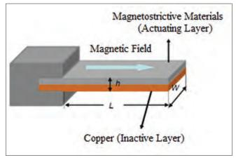
Figure 5: Magnetostrictive milli/micro-cantilever cantilever structure
