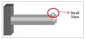
Figure 16: Point mass located at the free end of cantilever beam<sup>[45]</sup>
