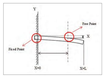
Figure 9: Deformation in Fixed-Free cantilever beam
