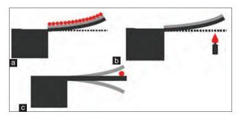
**Figure 3:** Sensor operating modes based on the cantilever. (a) Static mode, (b) heat mode, (c) dynamics mode<sup>[34]</sup>
