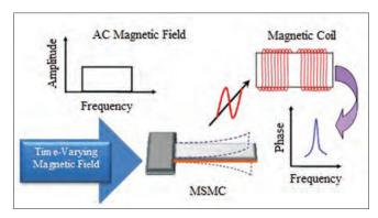
**Figure 6:** Magnetostrictive milli/micro-cantilever performance as a convertor for biological sensors<sup>[44]</sup>
