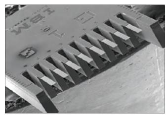
Figure 4: Scanning electron microscope image of an array of cantilever sensor<sup>[40]</sup>
