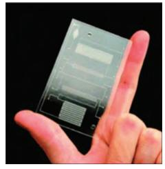
Figure 2: Laboratory on chip for bacteria detection[19]
