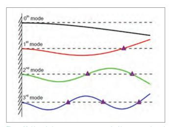
**Figure 11:** Natural vibration motions at zero to third harmonic modes and the nodes related to cantilever beam<sup>[47]</sup>
