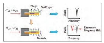
**Figure 8:** Magnetostrictive milli/micro-cantilever (MSMC) performance as biological sensor for bacteria detection. Bacteria connection is done on both sides of MSMC<sup>[44]</sup>
