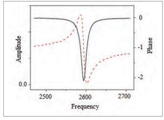
**Figure 14:** Resonant spectrum (curves of phase and amplitude signals according to frequency) for the main mode in magnetostrictive milli/micro-cantilever with the dimensions of 3.0 mm  $\times$  1.0 mm  $\times$  35 mm<sup>[39]</sup>
