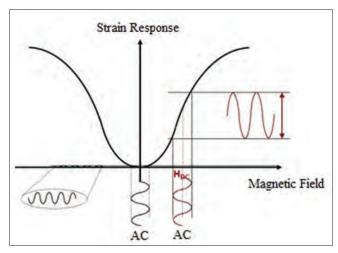
Figure 7: Magnetic material's magnetic response in magnetostrictive milli/micro-cantilever under the influence of external magnetic field
