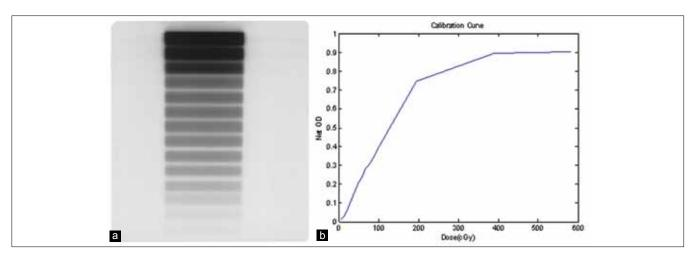
Figure 2: The extended dose range film calibration, (a) the exposed film, (b) calibration plot
