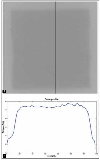
Figure 8: The profile results for 18 MV beam by film dosimetry, (a) extended dose range 2 film, (b) profile of corresponding line
