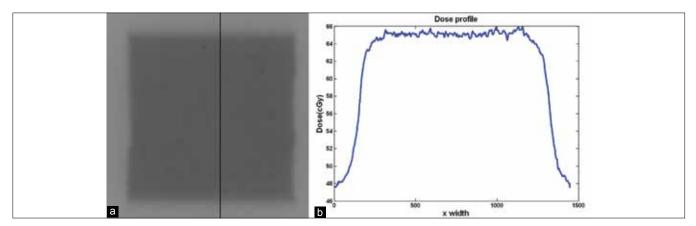
Figure 5: The profile of film dosimetry in 6 MV beam, (a) extended dose range 2 film, (b) profile of corresponding line
