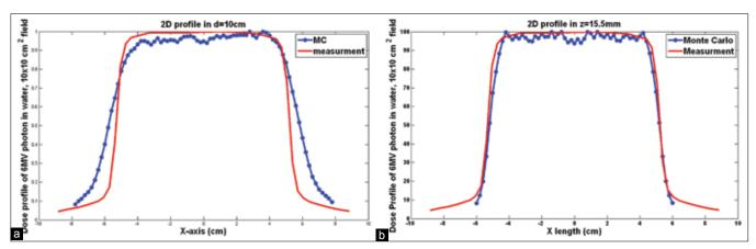
Figure 4: Profile results at 6 MV, (a) 6.5 MeV and full width of half maximum (FWHM) 0.2, (b) 6.5 MeV and FWHM 0.3
