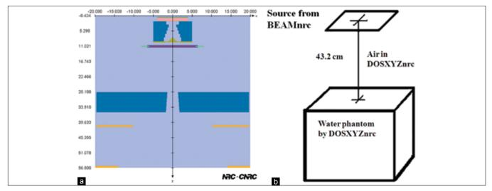
Figure 1: the schematic of simulation; (a) the simulated schematic of ONCOR linac (X-Z view) and (b) simulated phantom in DOSXYZnrc
