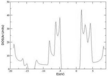
Figure 8: Density of states for SiC calculated by DFTB+ using the parameterization set pbc-0-3
