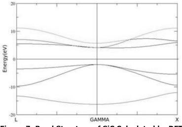
Figure 7: Band Structure of SiC Calculated by DFTB+ along L- Gamma-X line using the parameterization set pbc-0-3
