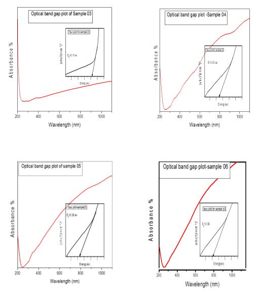
Figure 4: UV-Vis spectra of Ba<sub>1-x</sub>Zr<sub>0.5x</sub>Al<sub>0.3</sub>Fe<sub>11.7</sub>O<sub>19</sub> (x=0.0, 0.1, 0.2, 0.3, 0.4, 0.5)
