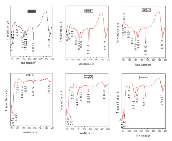
Figure 3.2: FTIR spectra for the samples  $Ba_{1-x}Zr_{0.5x}Al_{0.3}Fe_{11.7}O_{19}$  (x=0.0, 0.1, 0.2, 0.3, 0.4, 0.5)
