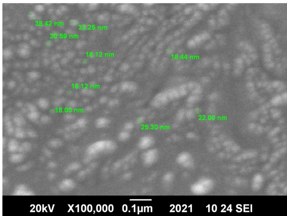
Figure 4: SEM image of the silver nanoparticles
