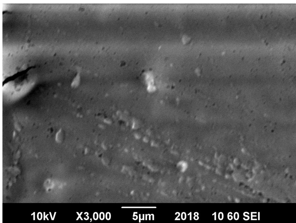
Figure 5: SEM image of Ag-PVA nanocomposite
