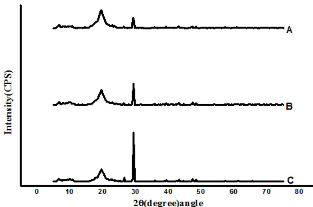
**Figure 1: XRD results of Ag-PVA nanocomposites of A: 1mg Ag NP, B: 3mg Ag NP and C: 5mg Ag NP**
