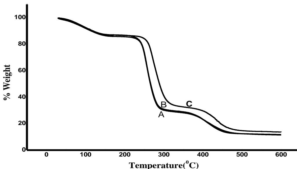
**Figure 2: TGA of Ag-PVA nanocomposites of A: 1mg Ag NP, B: 3mg Ag NP and C: 5mg Ag NP**
