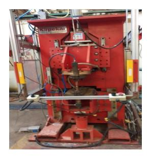
Figure 1. Kirperker RSW welding machine
