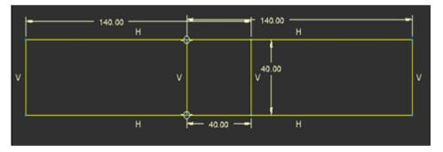
Figure 2. Dimension of specimen
