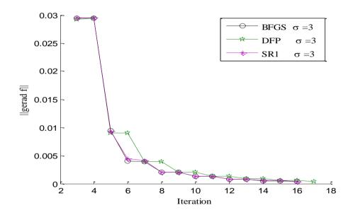
Figure 17. Trend for reduction of  $\|\vec{\nabla f}\|$  after each iteration of VMM cycle with  $\sigma = 3$  (the step heat flux)
