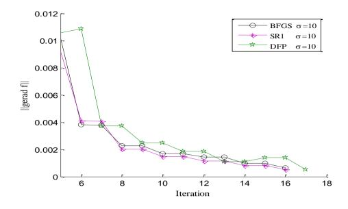
Figure 18. Trend for reduction of  $\|\overline{\nabla f}\|$  after each iteration of VMM cycle with  $\sigma = 10$  (the step heat flux)
