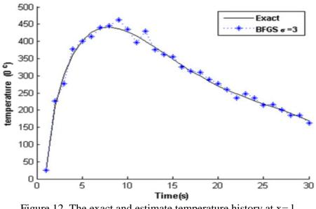
Figure 12. The exact and estimate temperature history at x=1 with  $\sigma = 3$  (the third degree polynomial heat flux).
