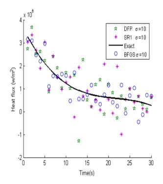
Figure 4. The estimation of the third degree polynomial heat Flux with  $\sigma = 10$
