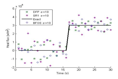
Figure 10. The estimation of the step heat flux with  $\sigma = 10$
