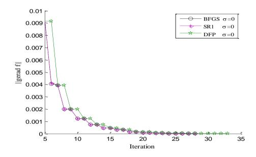
Figure 16. Trend for reduction of  $\|\overrightarrow{\nabla f}\|$  after each iteration of VMM cycle with  $\sigma = 0$  (the step heat flux).
