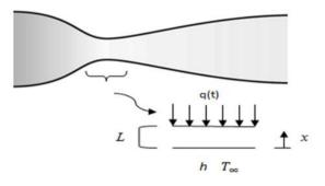
Figure 1. The one-dimensional rocket nuzzle throat geometry
