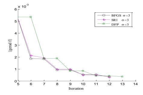
Figure 14. Trend for reduction of  $\|\overrightarrow{\nabla f}\|$  after each iteration of VMM cycle with  $\sigma = 3$  (the third degree polynomial heat flux).
