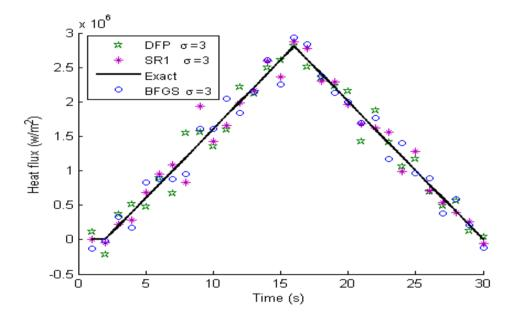
Figure 6. The estimation of the triangular heat flux with  $\sigma = 3$
