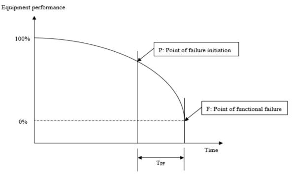
Figure 3. P-F interval (Rausand, 1998)
