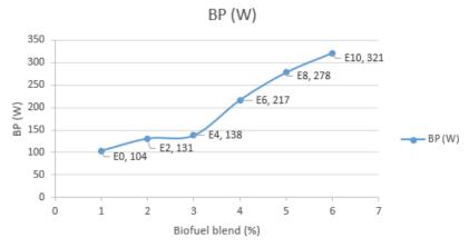
Figure 6: Engine performance on brake power (W) with biofuel blend (%)
