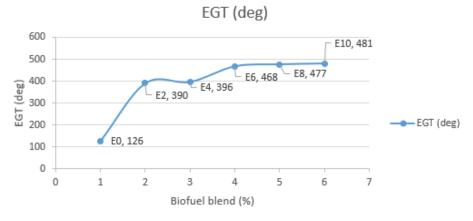
Figure 5: EGT ( $^{\circ}C$ ) of the biofuel blend (%)
