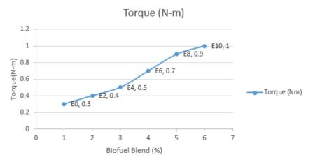
Figure 4: The engine torque (N/m) with ethanol blend (%)
