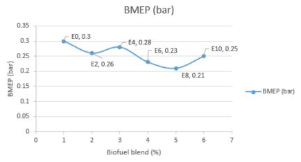
Figure 7: The BMEP (bar) of an engine with different ethanol blend (%)
