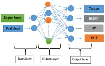
Figure 3: Artificial neural network for predicting engine performance characteristics of biofuel
