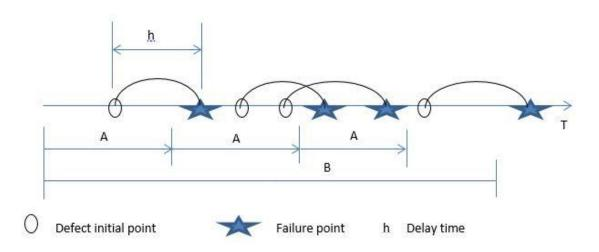
Figure 1. Delay time concept showing a defect's initial points and failure points
