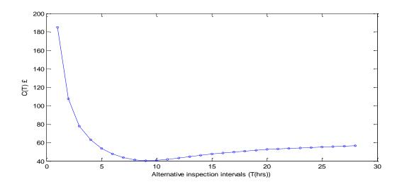
Figure 2. Inspection interval and cost effect
