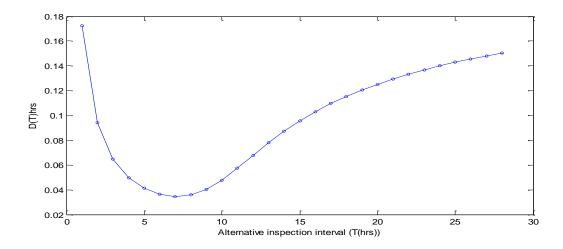
Figure 3. Inspection interval and downtime effect
