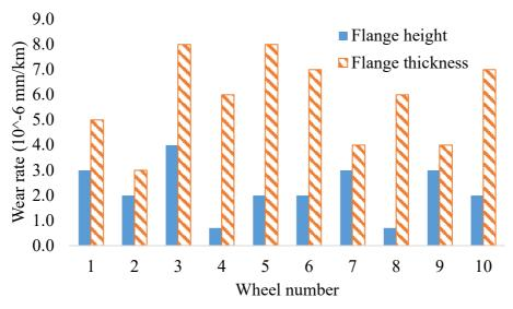
Figure 24: Wear rate of right flange height and thickness
