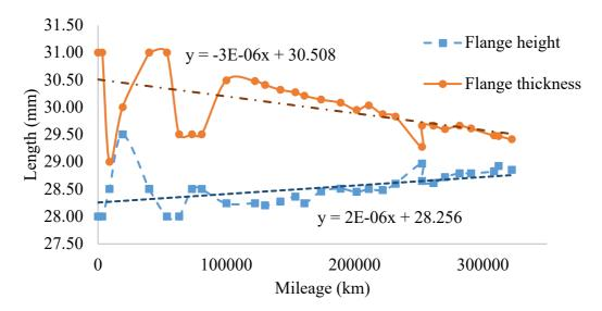
Figure 5: Railway wheel profile data for wheel 2R
