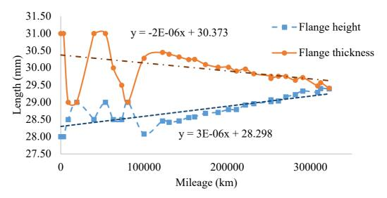
Figure 19: Railway wheel profile data for wheel 6L
