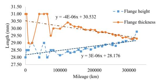
Figure 10: Railway wheel profile data for wheel 7R
