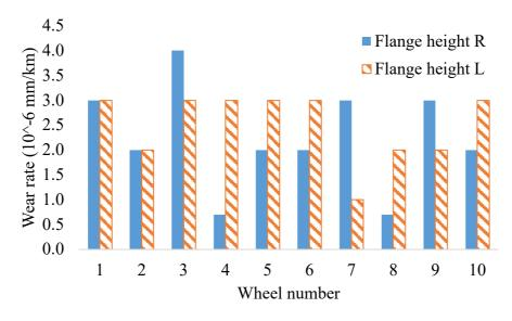
Figure 28: Wear rate of flange height
