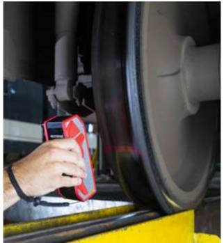
Figure 2: Calipri wheel measurement device
