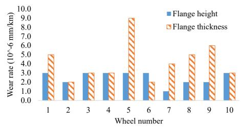
Figure 25: Wear rate of left flange height and thickness
