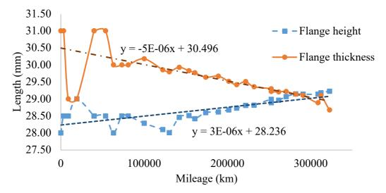
Figure 14: Railway wheel profile data for wheel 1L
