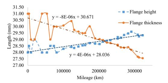
Figure 6: Railway wheel profile data for wheel 3R
