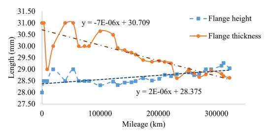
Figure 9: Railway wheel profile data for wheel 6R
