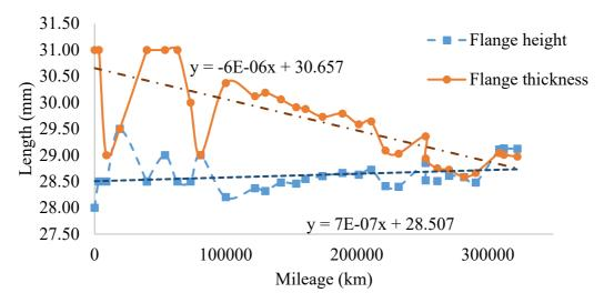
Figure 11: Railway wheel profile data for wheel 8R
