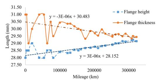
Figure 16: Railway wheel profile data for wheel 3L
