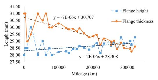
Figure 13: Railway wheel profile data for wheel 10R
