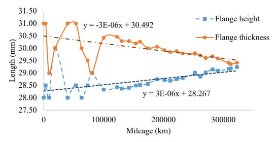
Figure 17: Railway wheel profile data for wheel 4L
