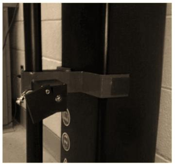
Figure 7: Lockout Device (Installed)
