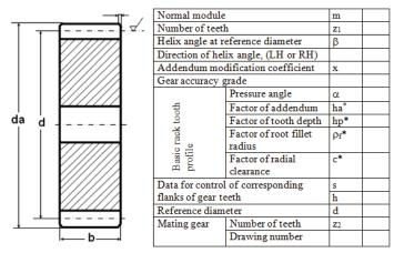
Figure 1. Typical data for gear drawings to be given by the gear designer for the gear manufacturer, according to NC 02-04-04: 78
