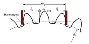
Figure 2. Measurement of base tangent length over 3 teeth in spur gear
