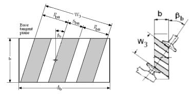
Figure 3. Measurement of base tangent length over 3 teeth in helical gear (top view)
