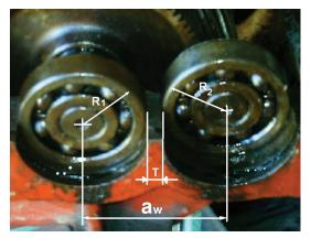
Figure 4. Parameters for calculation of centre distance (aw) by means of center holes distance or bearing housing bores radii (R1 + R2) plus the distance (T) between them
