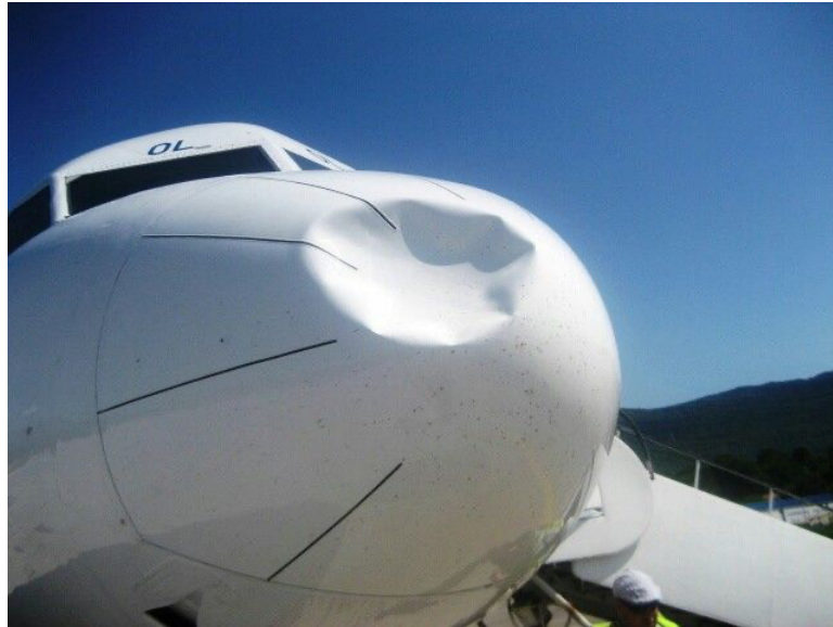
Figure 1 : Montenegro airlines Fokker 100 bird strike nosecone damage (Discover ideas about Montenegro Airlines, 2016)
