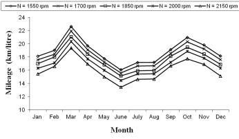
Figure 4. Monthwise car mileage at different speeds
