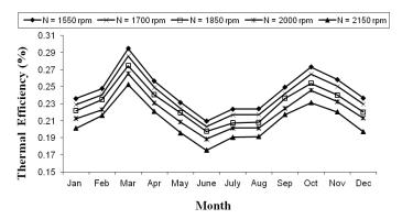
Figure 3. Monthwise car thermal efficiency at different speeds
