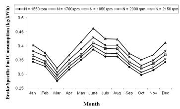
Figure 5. Monthwise car brake specific fuel consumption at different speeds
