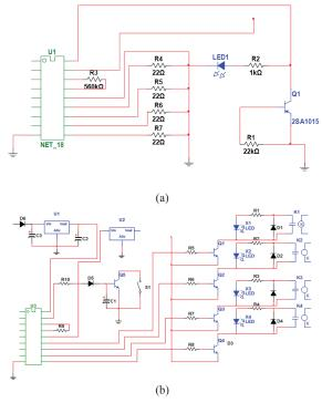
Figure 1. Transmitter (a) and receiver schematic diagrams (b)
