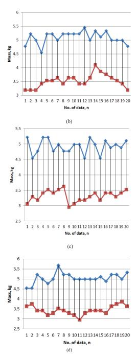
Figure 3. Load during gears' engage (♠) and disengage (■) for first gear (a), second gear(b), third gear(c) and fourth gear (d).
