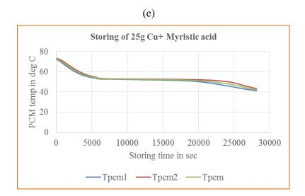
Figure 12 (a) Storing time vs PCM temp of 5g Cu added in Paraffin Wax (b) Storing time vs PCM temp of 5g Cu added in Myristic acid (c) Storing time vs PCM temp of 15g Cu added in Paraffin Wax (d) Storing time vs PCM temp of 15g Cu added in Myristic acid (e) Storing time vs PCM temp of 25g Cu added in Paraffin Wax (f) Storing time vs PCM temp of 25g Cu added in Myristic acid
