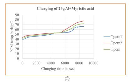
Figure 6 Charging time vs PCM temp of 5g Al added in Paraffin Wax (a) Charging time vs PCM temp of 5g Al added in Myristic acid (b) Charging time vs PCM temp of 15g Al added in Paraffin Wax (c) Charging time vs PCM temp of 15g Al added in Myristic acid (d) Charging time vs PCM temp of 25g Al added in Paraffin Wax (e) Charging time vs PCM temp of 25g Al added in Myristic acid(f)
