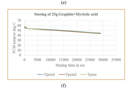
Figure 10 Storing time vs PCM temp of 5g Graphite added in Paraffin Wax (a) Storing time vs PCM temp of 5g Graphite added in Myristic acid (b) Storing time vs PCM temp of 15g Graphite added in Paraffin Wax (c) Storing time vs PCM temp of 15g Graphite added in Myristic acid (d) Storing time vs PCM temp of 25g Graphite added in Paraffin Wax (e) Storing time vs PCM temp of 25g Graphite added in Myristic acid (f).
