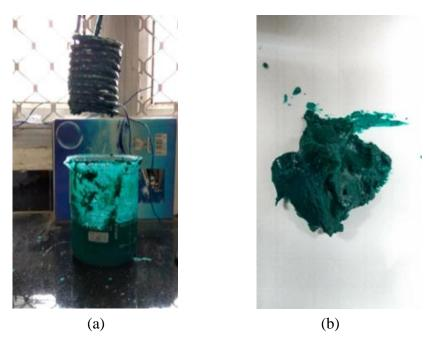
Figure 8. 25g Cu added Myristic acid after 3h 30 minutes (a) 25g Cu Myristic acid paste (b).
