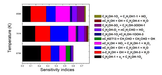
Figure 9. Main first-order sensitivity indices for simulated *n*-butanol ignition delays with respect to reaction rates at selected temperatures and pressures. The shading for each reaction is shown in the legend. P = 20 bar,  $\phi = 1$ .
