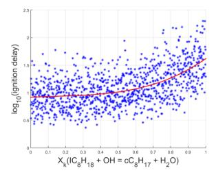
Figure 4. HDMR component functions (solid line) of simulated TRF ignition delays shown on-top of the scatter. P = 20 bar,  $\phi = 1$ , T = 761 K. Sensitivity with respect to  $IC_8H_{18} + OH = cC_8H_{17} + H_2O$ .
