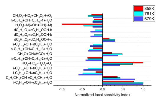
Figure 17. Brute-force local sensitivity result based on updated mechanism for TRF mixtures at P = 20 bar,  $\phi = 1$ .
