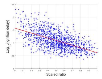
Figure 5. Scatter plot and HDMR component function for predicted log (ignition delay) of TRF against the scaled branching ratio for the two iso-octane main H abstraction reactions T = 761 K,  $\phi = 1$ , P = 20 bar.
