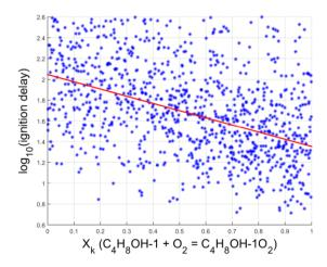
Figure 12. Component function for *n*-butanol mixture at 679 K with respect to  $C_4H_8OH-1+O_2=C_4H_8OH-1O_2$ .
