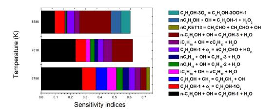
Figure 8. Main first-order sensitivity indices for simulated TRF/n-butanol ignition delays with respect to reaction rates at selected temperatures and pressures. The shading for each reaction is shown in the legend. P = 20 bar,  $\phi = 1$ .
