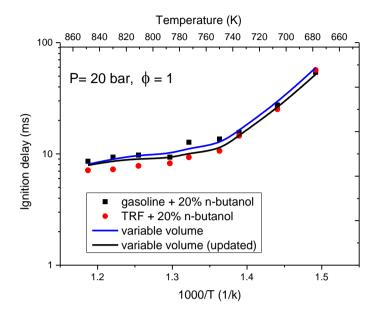
Figure 16. Ignition delay simulations showing how the updated mechanism compares with original LLNL data, TRF, n-butanol blend at P = 20 bar,  $\phi = 1$ .
