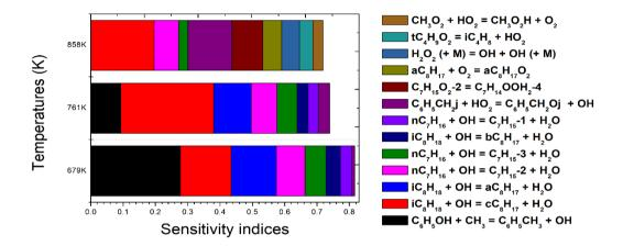
Figure 2. Main first-order sensitivity indices for simulated ignition delays of TRF at  $\phi$ =1 and P = 20 bar with respect to the key reaction rates at selected temperatures and pressures.
