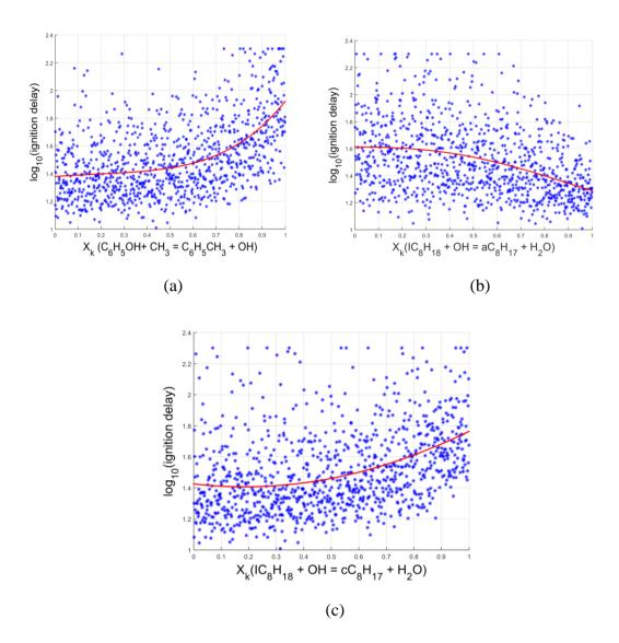
Figure 3. HDMR component functions (solid line) of simulated TRF ignition delays shown on-top of the scatter. P=20 bar,  $\phi=1$ , T=679 K. Sensitivity with respect to (a) CH3 + C<sub>6</sub>H<sub>5</sub>OH = C<sub>6</sub>H<sub>5</sub>CH<sub>3</sub> + OH (b) IC<sub>8</sub>H<sub>18</sub> + OH = aC<sub>8</sub>H<sub>17</sub> + H<sub>2</sub>O (c) IC<sub>8</sub>H<sub>18</sub> + OH = cC<sub>8</sub>H<sub>17</sub> + H<sub>2</sub>O.
