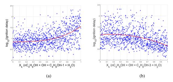
Figure 10. Component function for TRF/n-butanol mixture at T = 761 K with respect to (a) n-C<sub>4</sub>H<sub>9</sub>OH + OH = C<sub>4</sub>H<sub>8</sub>OH-1 + H<sub>2</sub>O (b) n-C<sub>4</sub>H<sub>9</sub>OH + OH = C<sub>4</sub>H<sub>8</sub>OH-3 + H<sub>2</sub>O.
