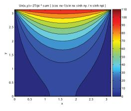
FIGURE 2 Temperature contour of thin square metal plate
