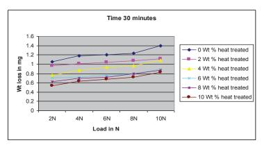
**FIGURE 10** Variation of weight loss with increase in load for Al6061 matrix alloy and Al 6061-Frit particulate composites under heat treatment conditions
