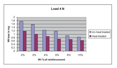
FIGURE 8 Variation of weight loss of Al6061 matrix alloy and 16061- Frit particulate composites.
