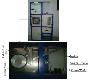
FIGURE 3 Photograph of sand abrasion testing apparatus
