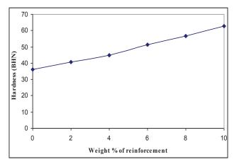
FIGURE 7 Variation of hardness with increase in weight % of reinforcement for as cast Al6061 matrix alloy and Al 6061-Frit particulate composites
