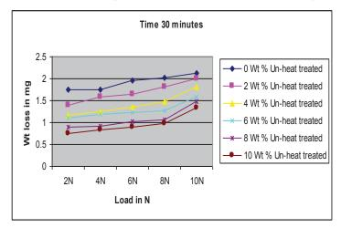
FIGURE 9 Variation of weight loss with increase in load for Al6061 matrix alloy and Al 6061-Frit particulate composites under un-heat treated conditions
