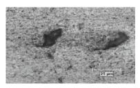
FIGURE 5 Optical micrograph of aluminium /frit composite indicating good bond between the matrix and frit particles.
