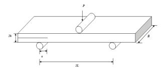
FIGURE 1 Schematic of the test configuration for the Mode II ENF Test.
