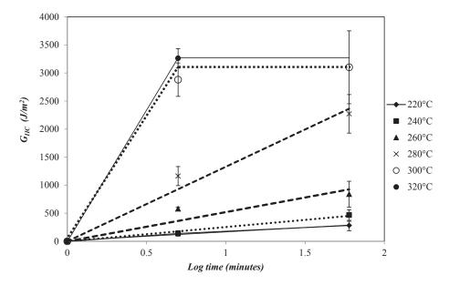
**FIGURE 5** Plot of  $G_{\text{IIC}}$  versus Log time
