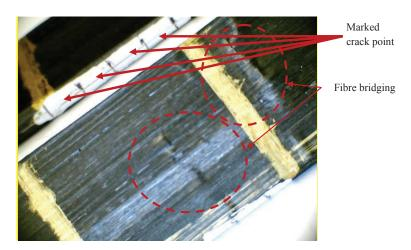
**FIGURE 9** Photograph of a mixed-mode test specimen showing fibre bridging as the crack propagates from the initial crack to the mid span position.
