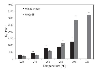
FIGURE 10 G<sub>c</sub> versus processing temperature following both Mode II and Mixed-Mode I/II Interlaminar Fracture tests on specimens manufactured using a dwell time of 5 minutes
