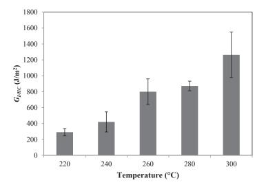
**FIGURE 6** Plot of G<sub>I/IIC</sub> at different processing temperatures for the Mixed-Mode fracture specimens manufactured using a dwell time of 5 minutes
