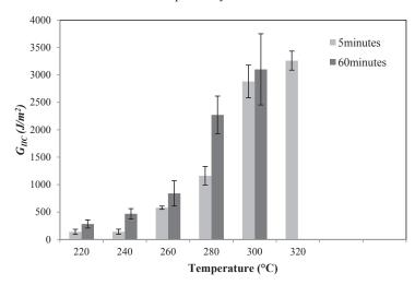
**FIGURE 4** Plot of G<sub>IIC</sub> as a function of processing temperature and dwell time.
