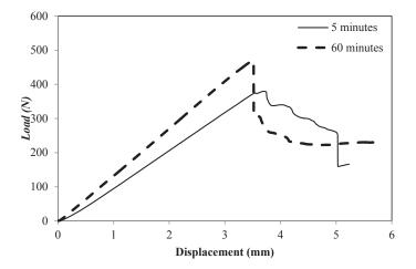
**FIGURE 7** (b) Typical MMF load-displacement traces following processing at 300° with dwell times of 5 and 60 minutes.
