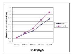
FIGURE 3 Load vs Heat lost to exhaust gas
