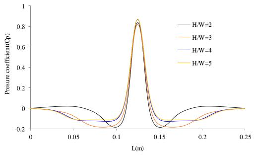
Figure 10. The wall pressure coefficients for Re = 500 and H/W = 2, H/W = 3, H/W = 4, and H/W = 5.
