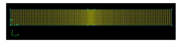
Figure 3. The mesh as built from Gambit
