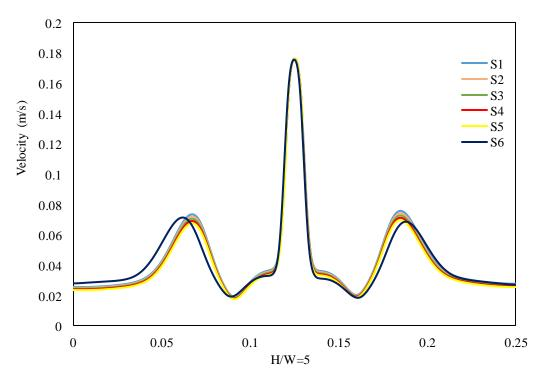
Figure 4. Plot of velocity for various mesh schemes for H/W=5
