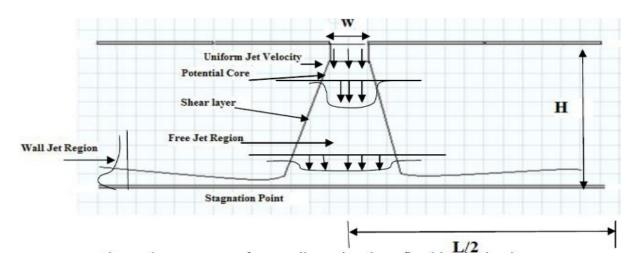
Figure 1. The geometry of a 2-D confined impinging jet
