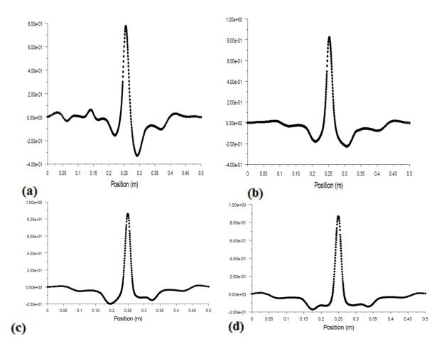
Figure 15. Normalized pressure coefficients for H/W=5, Re=750 and (a) t=0 s (b) t=2 s (c) t=4 s and (d) t=6 s in the unsteady regime
