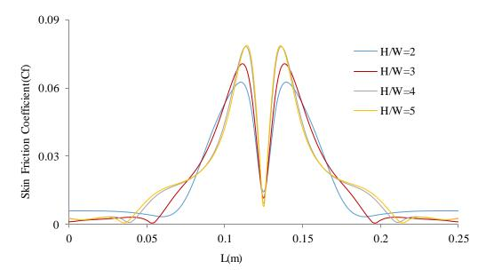
Figure 11. Target Wall friction coefficient for Re = 500 and H/W = 2, H/W = 3, H/W = 4, and H/W = 5.
