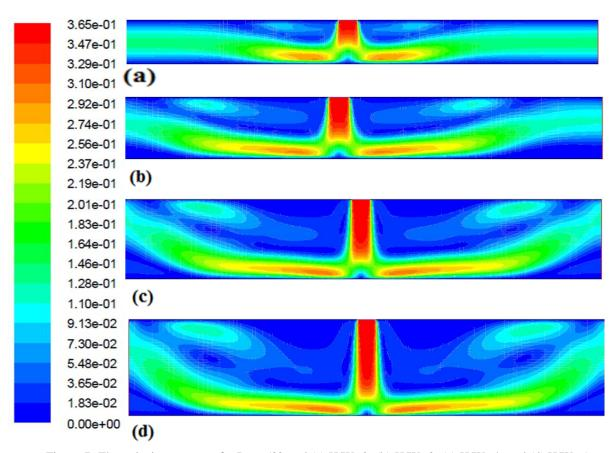
Figure 7. The velocity contours for Re = 500 and (a) H/W=2, (b) H/W=3, (c) H/W=4, and (d) H/W=5
