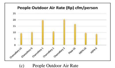
Figure 4. Average Fresh Air Flow (cfm) for each building blocks, Occupancy Number and People Outdoor Air Rate (Rp) cfm/person
