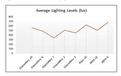
Figure 7. Average Electric Lighting Illumination Levels
