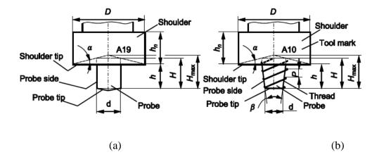
Figure 4. FSW tool (a) conical shoulder with flat pin (b) conical shoulder with conical pin,  $D=R_p$  and  $d=R_s$  (Roy et al., 2006) ISSN: 2180-1053 Vol. 10 No.1 January – June 2017 37
