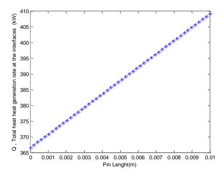
Figure 8. Variations total heat generation rate at the interfaces with pin length.
