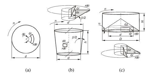
Figure 3. Active surfaces in FSW: (a) pin tip, (b) pin side, (c) shoulder tip
