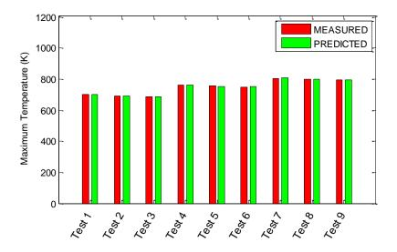
Figure 16. Bar chart for comparison of results for maximum temperature in Aluminum alloyISSN: 2180-1053Vol. 10 No.1January – June 201753
