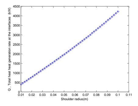
Figure 7. Variations total heat generation rate at the interfaces with shoulder radius
