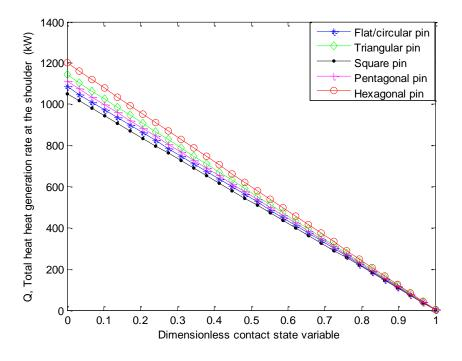
Figure 6. Effects of pin shape on the total heat generation rate at the interfaces
