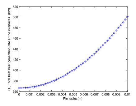
Figure 9. Variations total heat generation rate at the interfaces with pin radius
