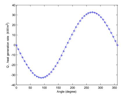
Figure 11. Variations heat generate with angle of rotation when the extent of sticking is 1 (full sticking condition)
