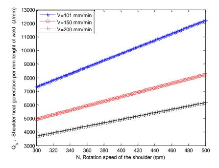
Figure 13. Effects of welding speed on the heat generation at the shoulder
