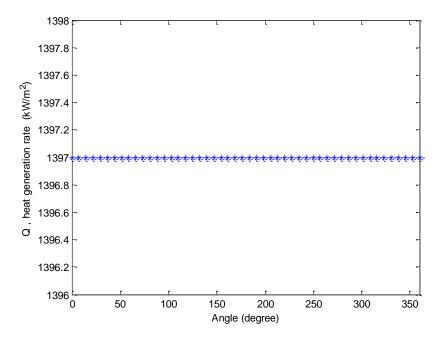
Figure 12. Variations heat generate with angle of rotation when the extent of sticking is 0 (full sliding condition)
