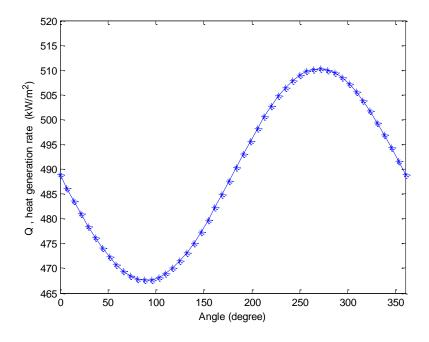
Figure 10. Variations heat generate with angle of rotation when the extent of sticking is 0.65
