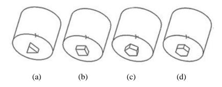
Figure 5. Different profiles pin used in FSW. (a) Triangular pin. (b) Square pin (c). Pentagonal pin. (d) Hexagonal pin
