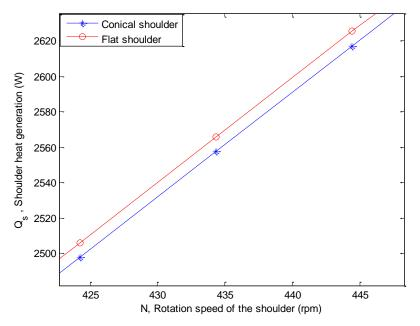
Figure 14. Effects of shoulder conical angle on the heat generation at the shoulder
