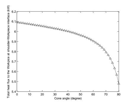
Figure 15. Effects of conical angle on the heat generation at the shoulder-workpiece interface
