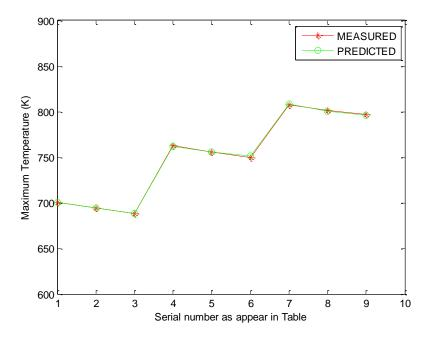
Figure 17. Line graph for comparison of results for maximum temperature in Aluminum alloy
