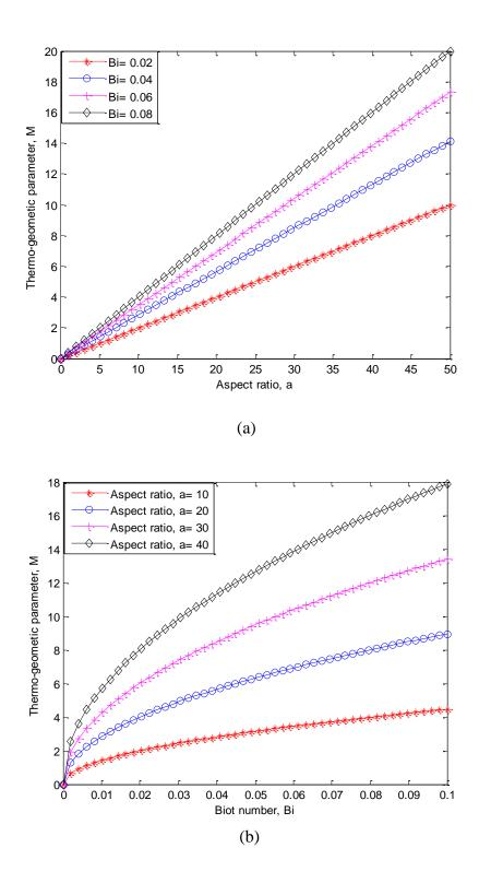
Figure 7. Effects of Biot number on the thermo-geometric parameter of the fin
