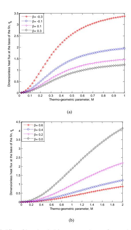
Figure 3. Effects of thermal conductivity parameter on heat transfer rate at the base of the fin
