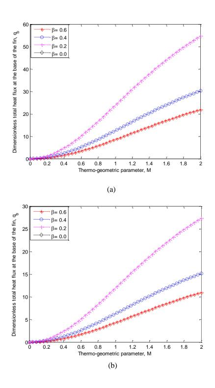
Figure 4. Effects of non-linear thermal conductivity parameter on the dimensionless total heat flux of the fin (a), Bi=0.04 (b) Bi=0.08
