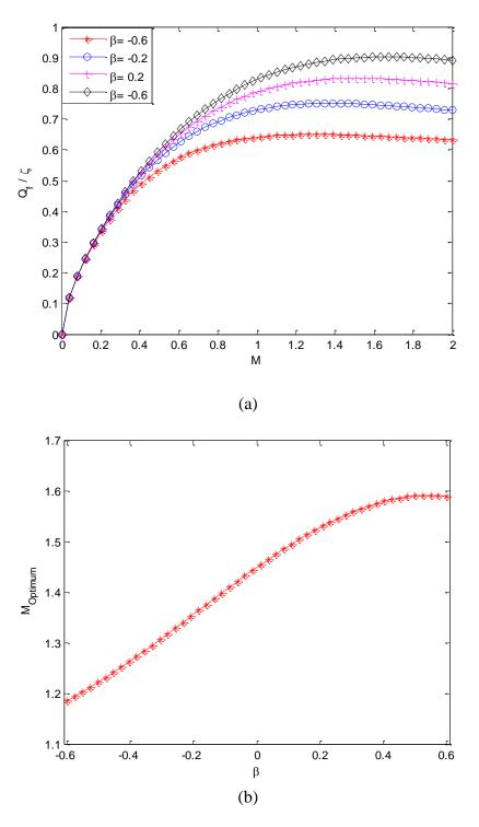
Figure 8 (a) Effects of non-linear thermal conductivity and thermo-geometric parameters on the dimensionless heat transfer,  $Q_f/\zeta$  (b) Effects of non-linear thermal conductivity parameter on the optimum thermo-geometric parameter
