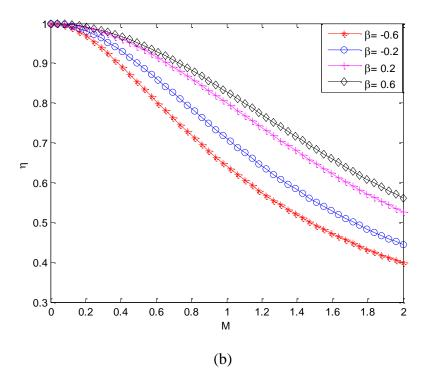
Figure 5. Effects of non-linear thermal conductivity and thermo-geometric parameters on the efficiency of the fin
