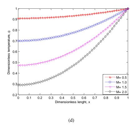
Figure 2. Effects of thermo-geometric parameter on the temperature distribution in the fin when (a)  $\beta$ = -0.3 (b)  $\beta$ =-0.1(c)  $\beta$ =0.1 (d)  $\beta$ =0.3
