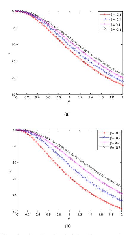
Figure 6. Effects of non-linear thermal conductivity and thermo-geometric parameters on the effectiveness of the fin
