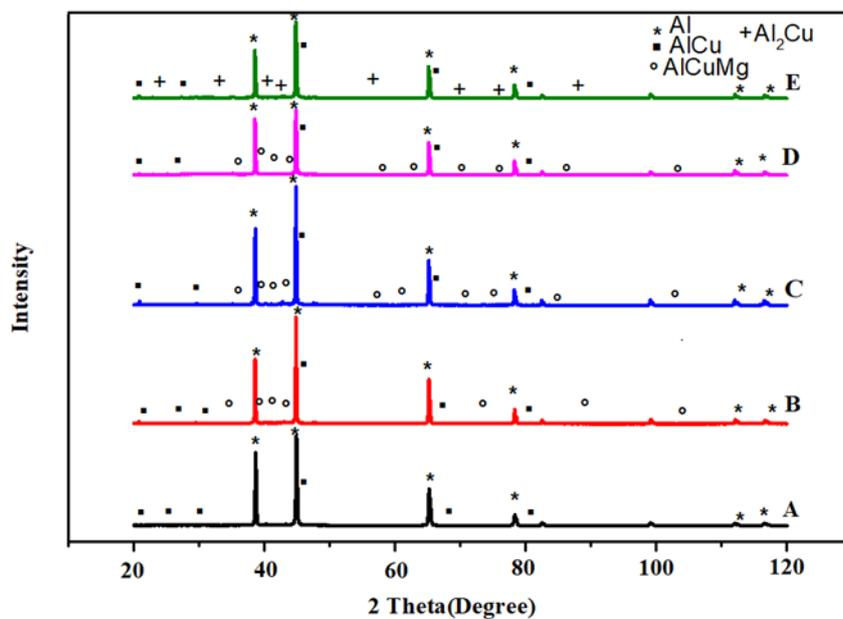
**Figure 4.** XRD of heat treated 2024 aluminum alloys; (A) control sample, (B) quenching sample, (C) homogenization sample, (D) artificial aging sample, and (E)recrystallization sample.
