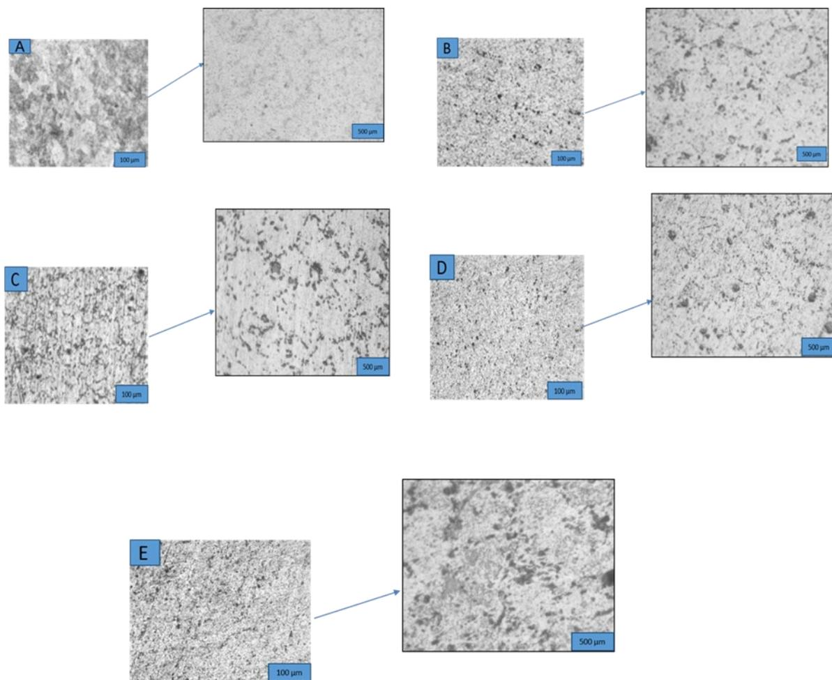
**Figure 2.** Micrographs of AA2024T3 materials: (A) control sample, (B) quenching sample, (C) homogenization sample, (D) artificial aging sample, and (E) recrystallization sample.
