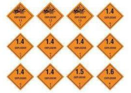
Figure 1. Label used for explosives according to IMDG code
